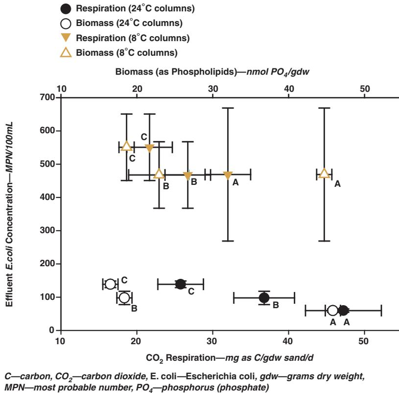
Influent concentration was 21,000 ± 6,000 MPN/100 mL for cold columns (8°C) and 19,000 ± 3,000 MPN/100 mL for warm columns (24°C). The vertical axis shows the effluent concentration; lower values indicate better removal. Letters correspond to column identification in Table 4.
