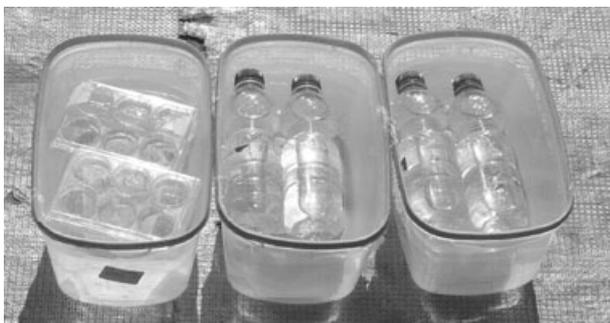
**Figure 2** *Escherichia coli* suspensions contained in transparent polystyrene six-well plates (on the left) and polyethylene terephthalate 300-ml bottles (centre and right) immersed in 3 l water baths, and exposed to strong natural sunlight on the laboratory roof in Southern Spain.
