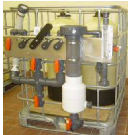
Figure 18: Tablet Chlorinator Secured by Two Hose Clamps to the Valve Assembly Bracket
