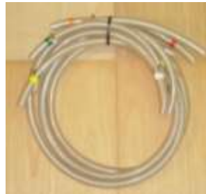
Figure 4: Color Coded Sections of 1-inch Braided Hose
