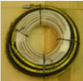
Figure 3: 1.5-inch Suction Hose and 1-inch Braided Hose
