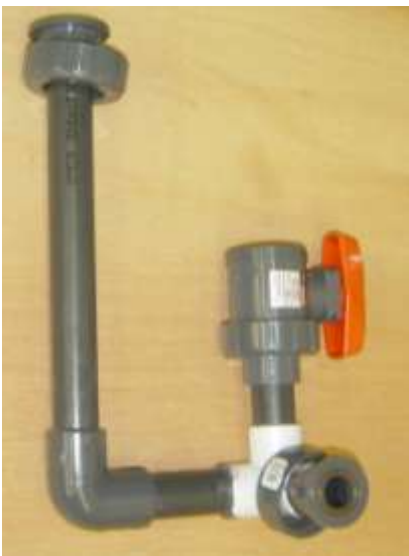
Figure 19: Chemical Injection Manifold
