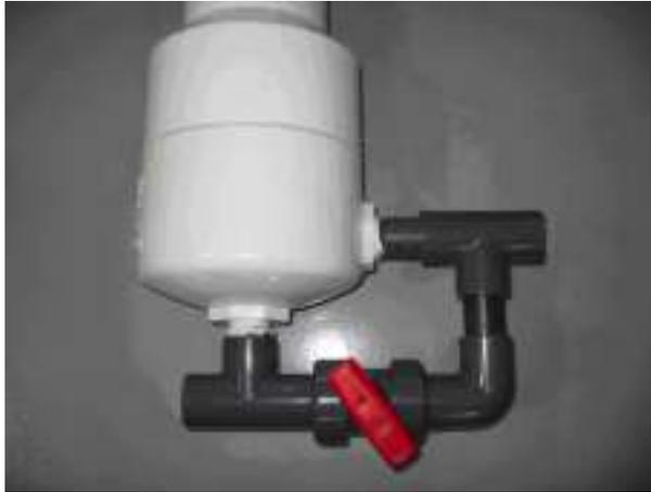
Figure 7. Chlorinator assembly
