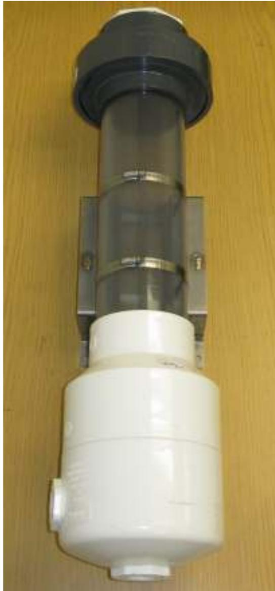
Figure 5. Mounted Chlorinator
